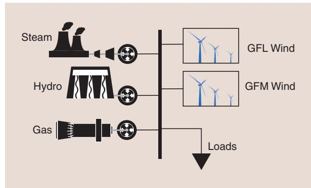
**Figure 12.** A simplified diagram of the test system with a combination of Type-4 GFL and GFM wind generation.
