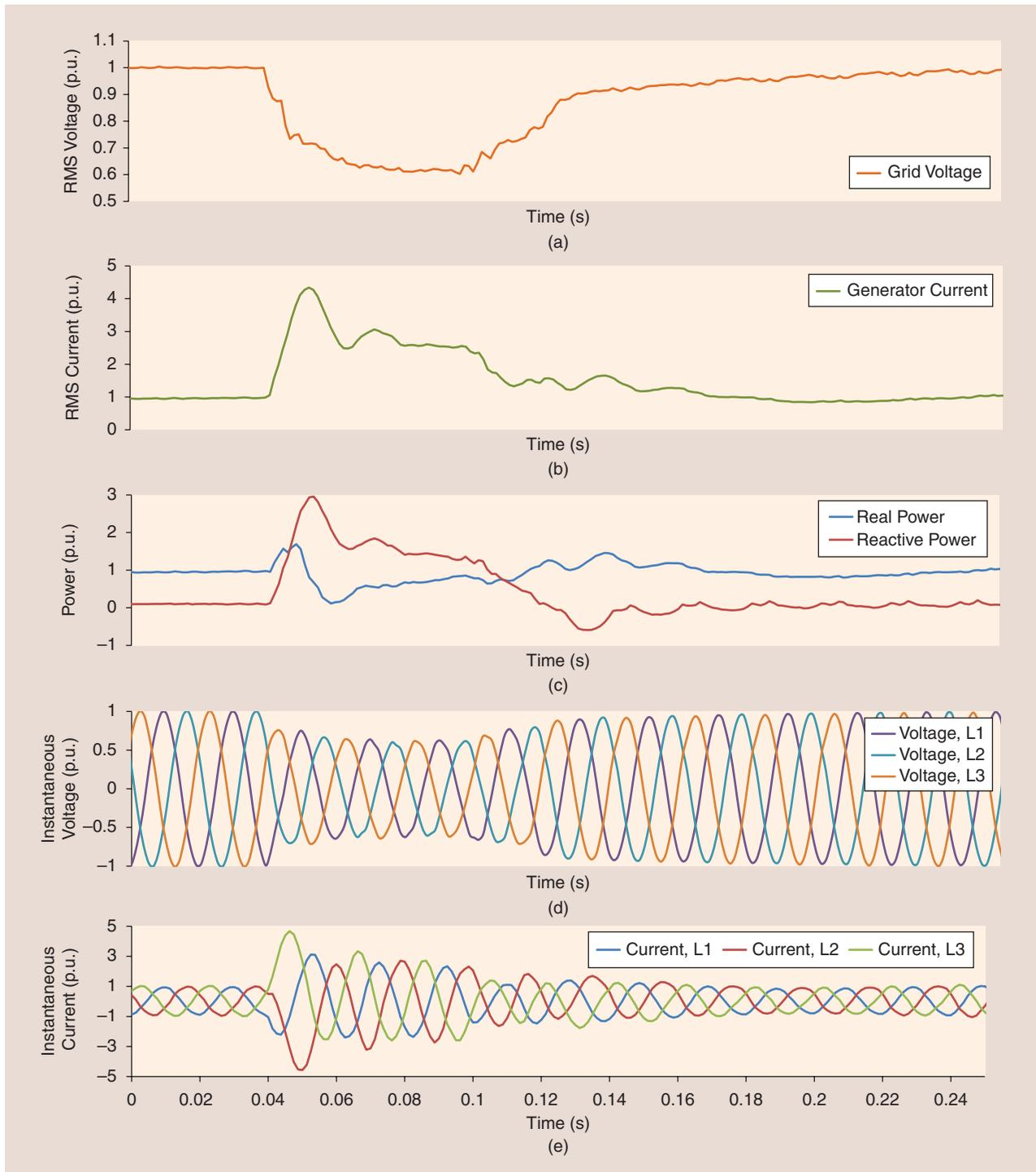
**Figure 11.** The measured voltage fault response of a Windflow 500 Type-5 wind turbine. p.u.: per unit; RMS: root mean square. (a) RMS voltage, (b) RMS current, (c) active and reactive power, (d) instantaneous voltage, and (e) instantaneous current.
