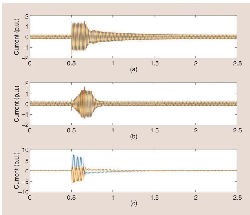
**Figure 6.** The ride-through performance of a GFM Type-4 wind turbine compared to a Type-5 one. p.u.: per unit. (a) A Type-4 grid-forming wind turbine, (b) Type-4 grid-following wind turbine, and (c) Type-5 wind turbine.
