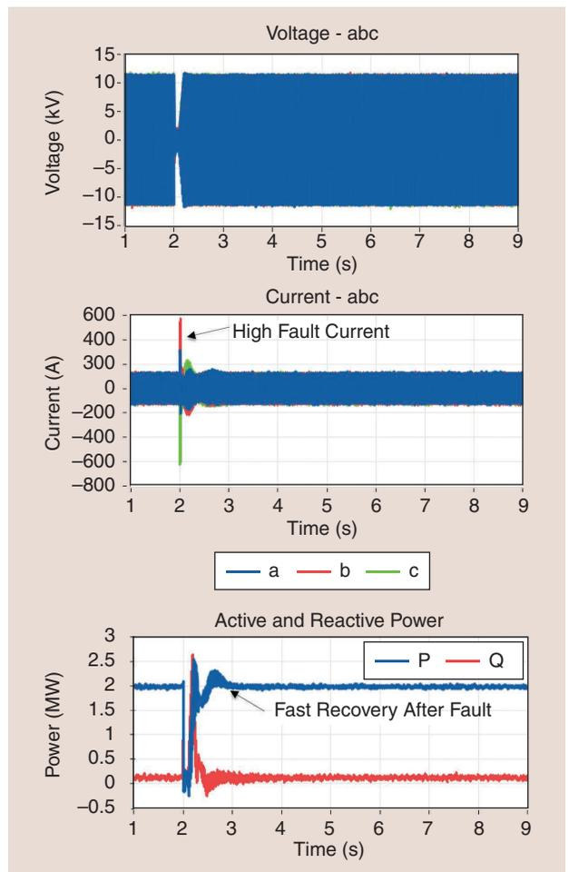
**Figure 9.** The measured fault ride-through of a 2-MW Type-3 GFM wind turbine.
