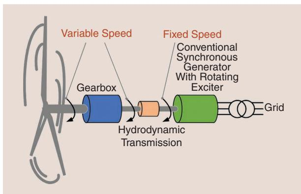
**Figure 3.** A Type-Va wind turbine with full-capacity hydrodynamic transmission.
