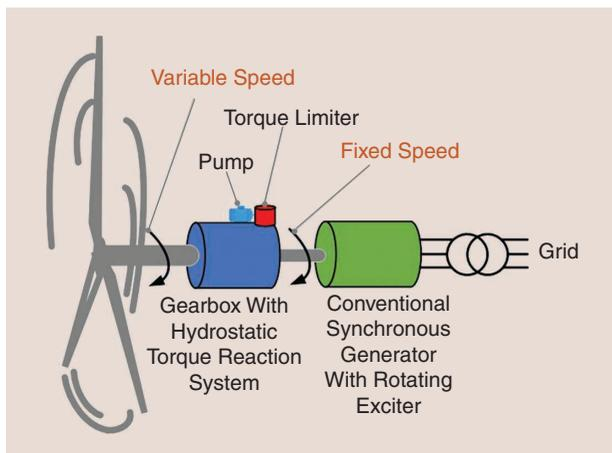
**Figure 4.** A Type-Vb wind turbine with a torque limiter and recently developed low-variable-speed system.
