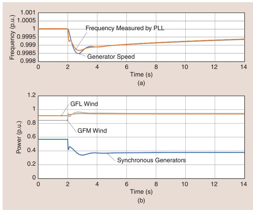
**Figure 14.** The system response to a loss of generation (66% GFL and 16% GFM wind). p.u.: per unit. (a) Frequency. (b) Power.
