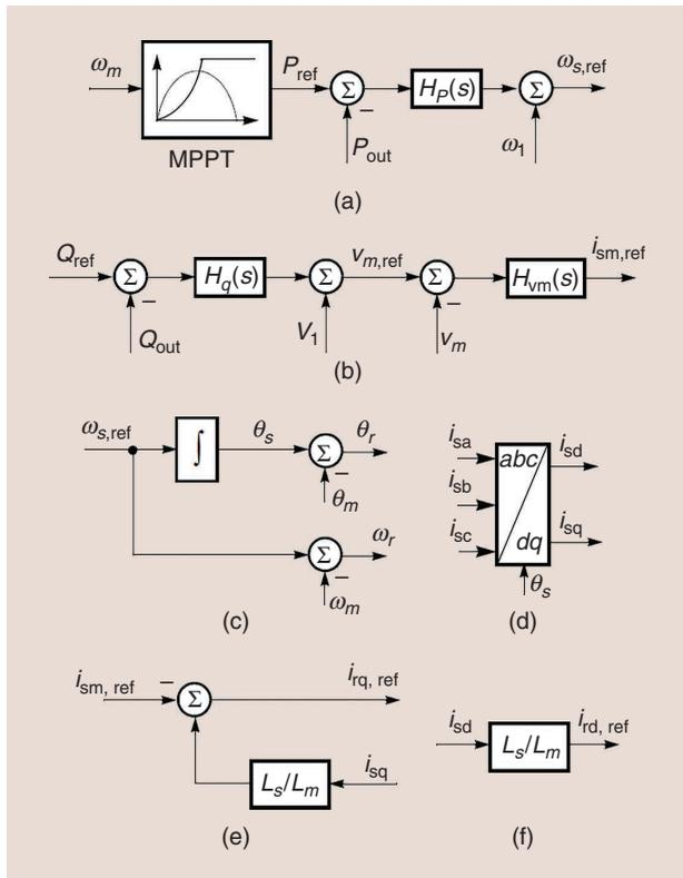
**Figure 8.** Outer control loops of the RSC for the GFM operation of a Type-3 wind turbine. MPPT: maximum power point tracking. (a) A turbine power controller. (b) A reactive power and voltage controller. (c) A phase angle reference signal. (d) A park transform for machine side converter. (e), (f) A rotor current control reference.
