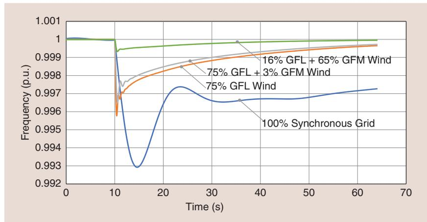
**Figure 13.** The frequency response of a test system for different combinations of Type-4 GFL and GFM wind generation. p.u.: per unit.
