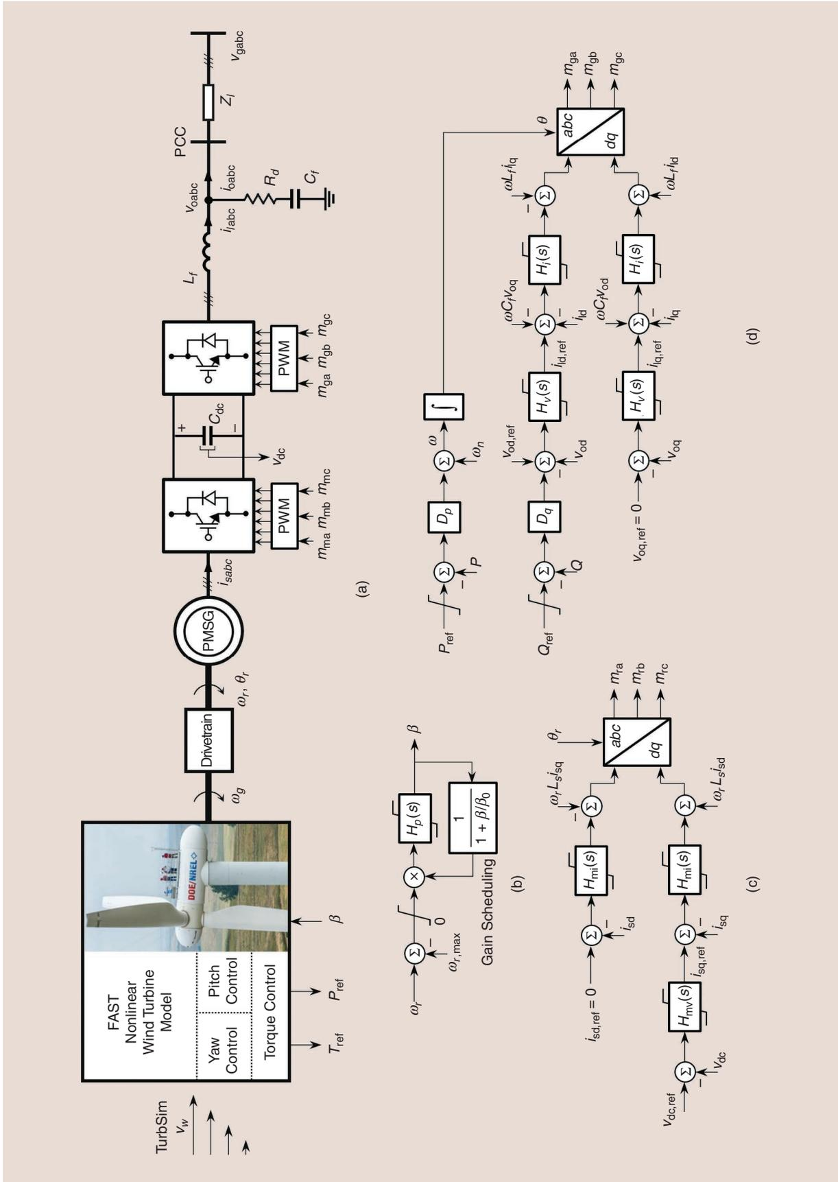
**Figure 5.** The GFM control for a Type-4 wind turbine generator. (a) The circuit diagram of the GFM-controlled Type-4 WTG. (b) The turbine patch control. (c) MSC control. (d) GFM GSC control (courtesy of NREL). GFM: grid forming; PMSG: permanent magnet synchronous generator; WTG: wind turbine generator; MSC: machine-side converter; GSC: grid-side converter.
