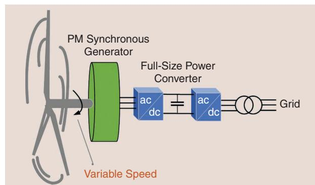
Figure 2. A Type-4 wind turbine topology. PM: permanent magnet.
