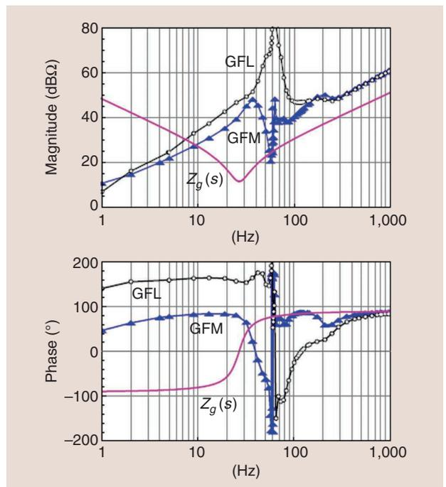
**Figure 10.** A comparison of the positive-sequence impedance response of a 2.5-MW Type-3 wind turbine in GFL and GFM modes.
