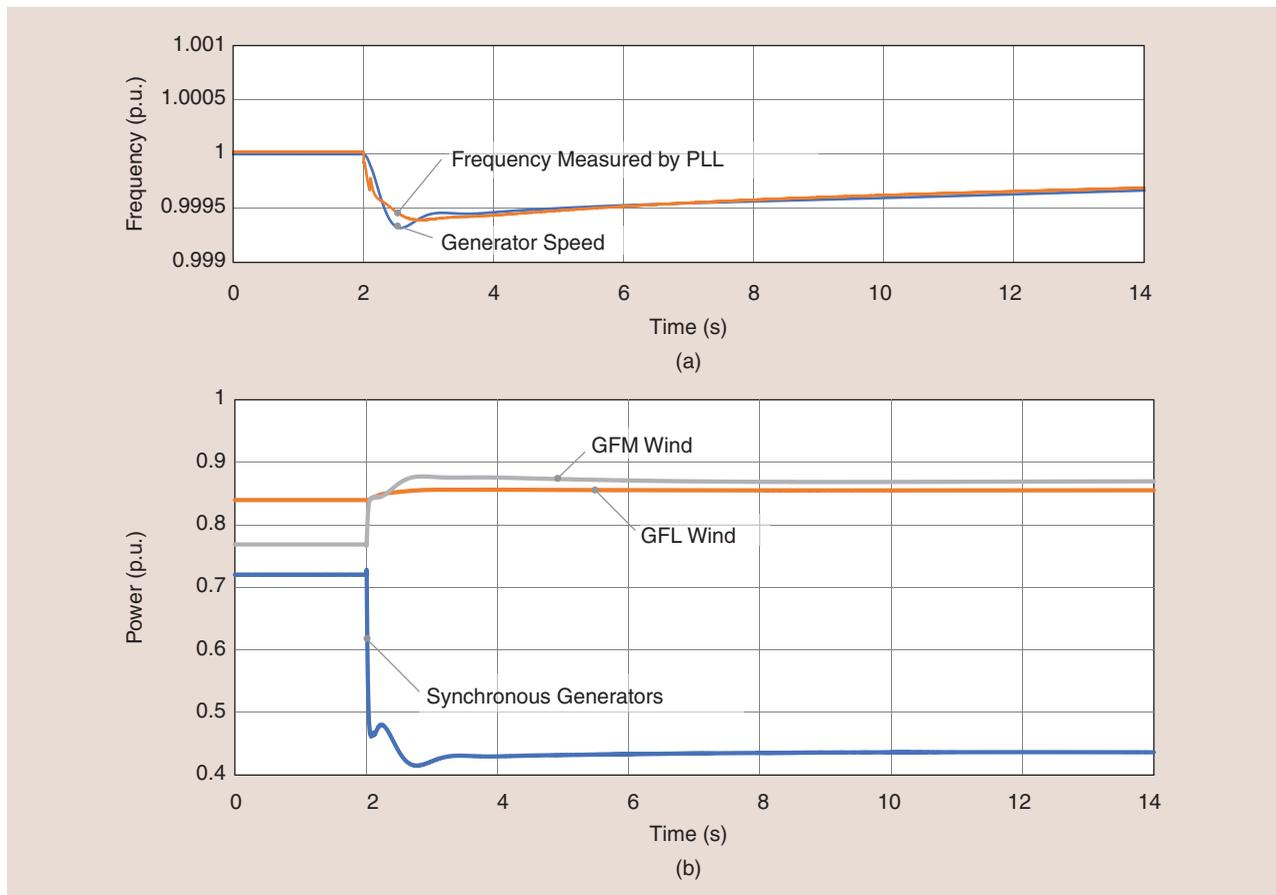
**Figure 15.** The system response to a loss of generation (16% GFL and 66% GFM wind). p.u.: per unit. (a) Frequency. (b) Power.
