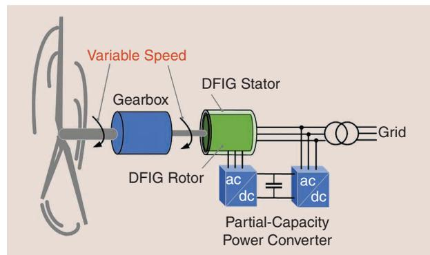
Figure 1. A Type-3 wind turbine topology.
